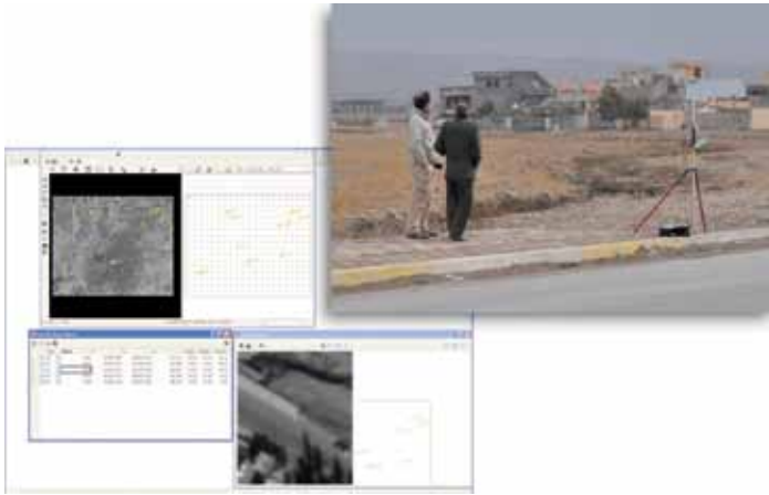
12 Fig. 3. Collecting the GCP (Ground Control Points) with differential GPS measurements
