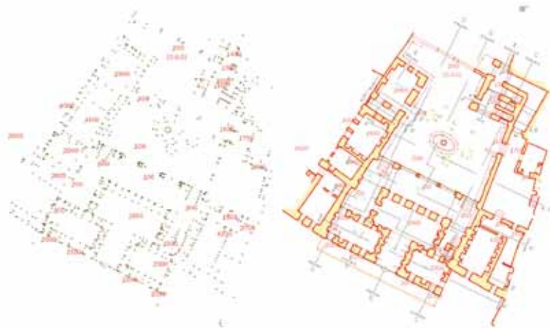
Fig. 1. Rashid Agha diwan khanah. Point acquisition and resulting plan view
